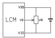
V<sub>DD~</sub>V<sub>0</sub>: LCD Driving voltage VR: 10k~20k
